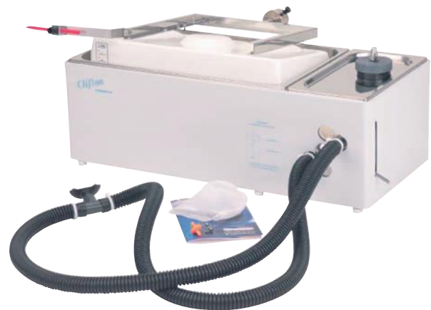
Figure 11.9 A spirometer. This instrument measures the volume of air breathed in and out of the lungs and can be used to measure oxygen consumption.
