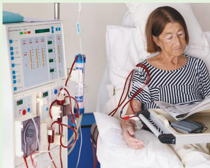
Figure 13.8 Kidney dialysis machine. The patient's blood is pumped to the dialyser, which removes urea and excess salts.
